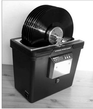
Our ultrasonic record cleaning device is simply constructed based on ready-made components available in DIY stores, and is designed for vinyl record lovers who are not satisfied with mechanical cleaners such as “Knosti”.
